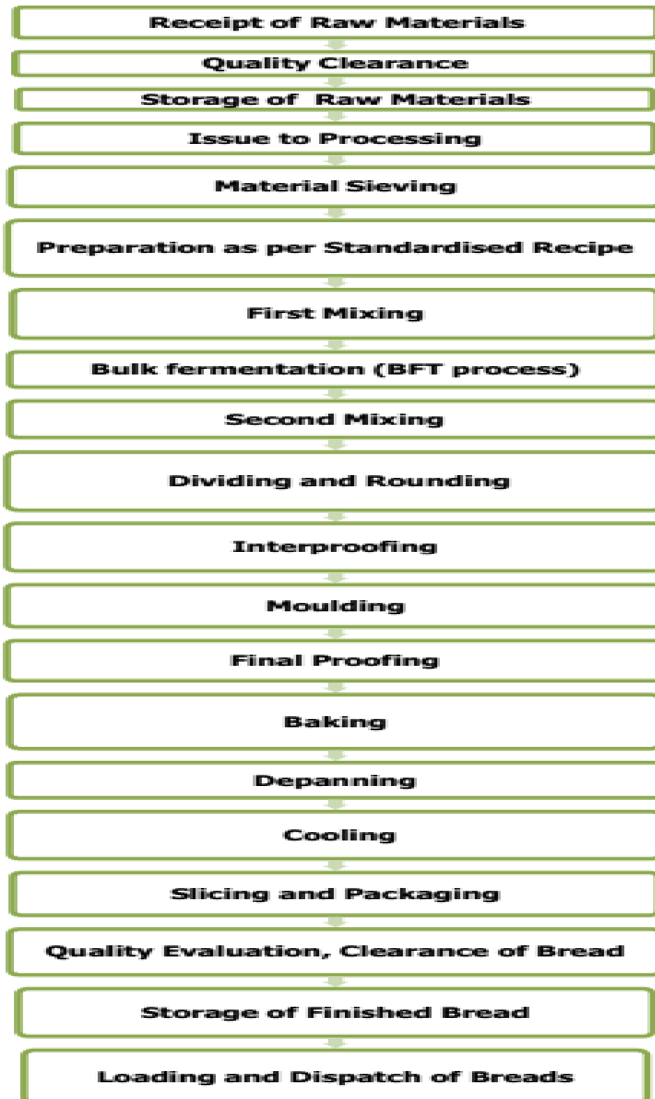
Figure 8: Process Flow Chart for Bread
